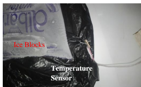
Figure 10: Temperature Sensor Close to an Ice Blocks
