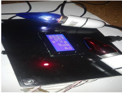
Figure 11: Blue Blub going on with the LCD Displaying the Fan's Status
